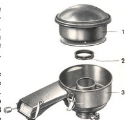
1 - Filter element, 2 - Gasket, 3 - Oil reservoir
