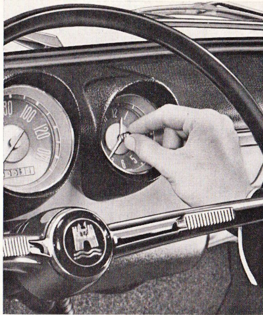
The Clock is electrically operated. The hands can be moved by turning the knob in the center of the dial.
