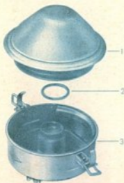
1-Filter element, 2-Gasket, 3-Oil reservoir
