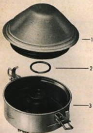
1-Filter element, 2-Gasket, 3-Oil reservoir
