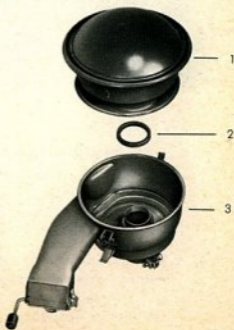
1 - Filter element, 2 - Gasket, 3 - Oil reservoir
