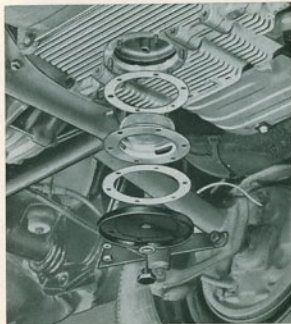
Cleaning the oil strainer.
