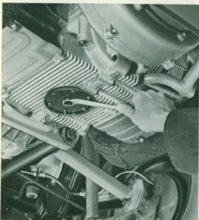
Draining the engine oil.
