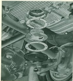
Cleaning the oil strainer.
