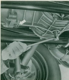
Draining the transmission oil.
