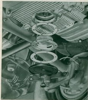
Cleaning the oil strainer.
