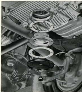
Cleaning the oil strainer.
