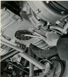
Draining the engine oil.
