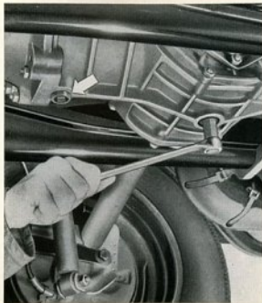
Draining the transmission oil.
