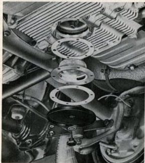
Cleaning the oil strainer.
