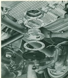
Cleaning the oil strainer.
