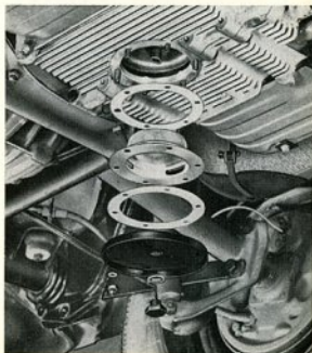
Cleaning the oil strainer.
