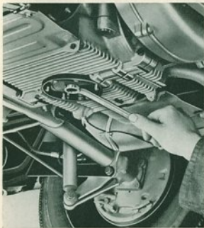
Draining the engine oil.
