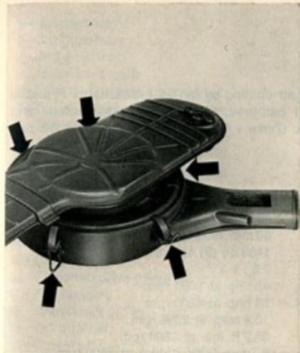
Clean lower part of cleaner carefully. The drain hole in the outer casing of the lower part must be clear.
