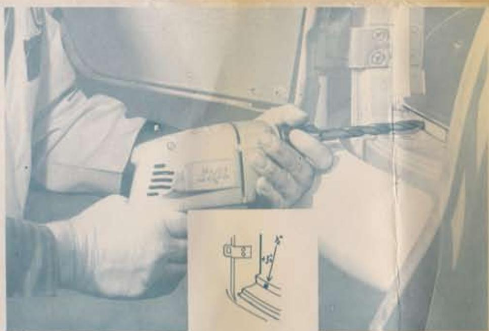
2 Pull the front door weather strip back along the bottom of the door frame. Drill a one half inch hole, three inches from center of hole to the hinge pillar of front door. Drill hole as low as possible. Punch one fourth inch hole in weather stripping. Be sure that the holes match up.
