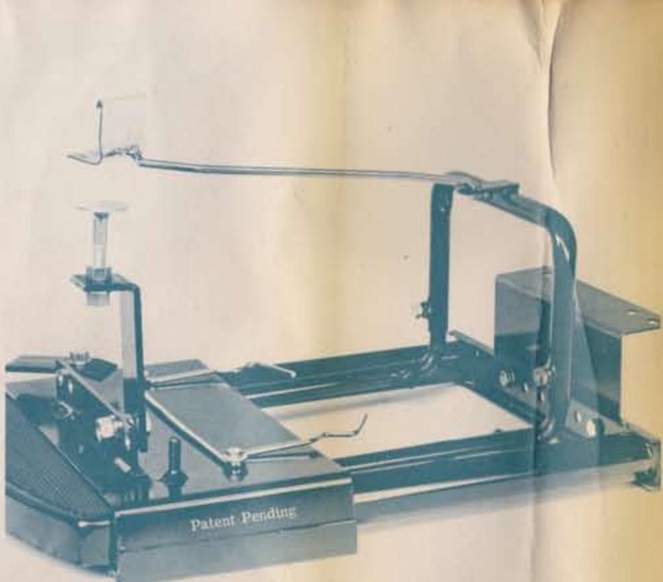
1 The Volkswagen step is a very simple accessory to install on any Volkswagen station wagon or truck. Slide the step from frame and apply a small amount of grease to the sliding tubes.
