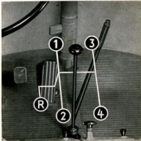
You now know how to "shift gears", and may at will shift to third and fourth positions. You will have noticed by now that the accelerator and clutch pedals are operated simultaneously, but in opposite directions. It is the coordination of these simultaneous operations that brings skill in shifting gears. To engage the **reverse gear**, first press down the gear lever vertically, move it to the left and pull it rearwards.
