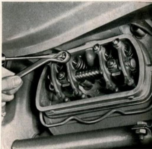
For this reason, **only adjust valve clearance when the engine is cold.**
