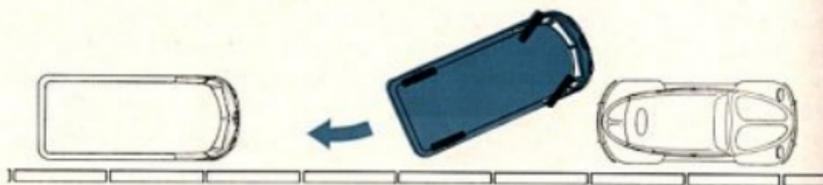
Now turn the steering wheel again to the right and pull up a little bit, until both ends of the vehicle come as close to the curb as possible.
