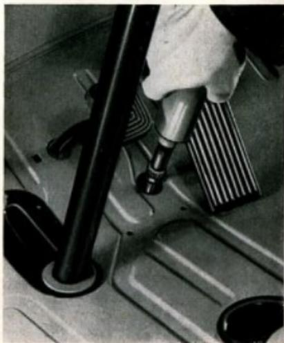
If the vehicle is driven mainly over rough roads, it is recommended to lubricate king pins and outer tie rod ends at more frequent intervals, say every 1000 km. (600 miles).
