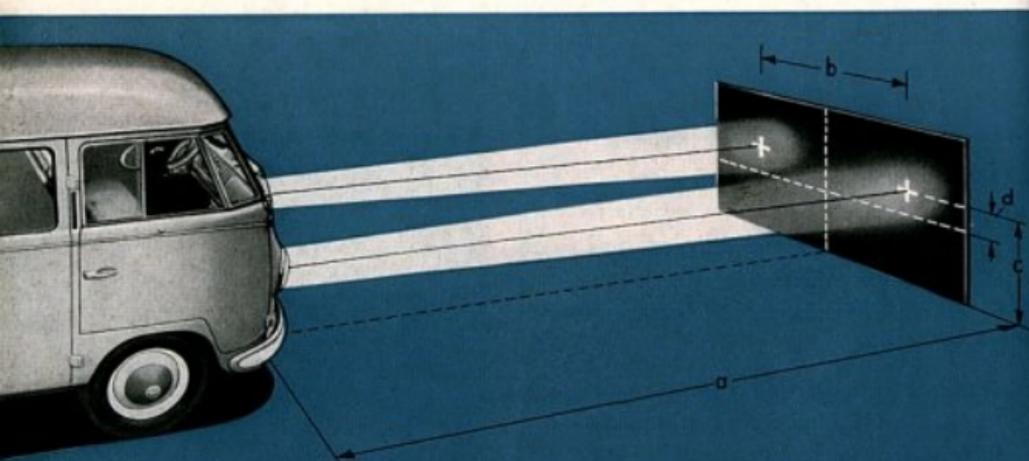
Dimensions:  $a = 5$  m. (16.4 ft.),  $b = 1100$  mm. (43.3 in.),  $c =$  Distance from floor to center point of headlamp lens,  $d = 50$  mm. (2 in.),  $d$  is the correct distance between the upper limit of the light spot and the center of the cross when adjusting the low (traffic) beam.
