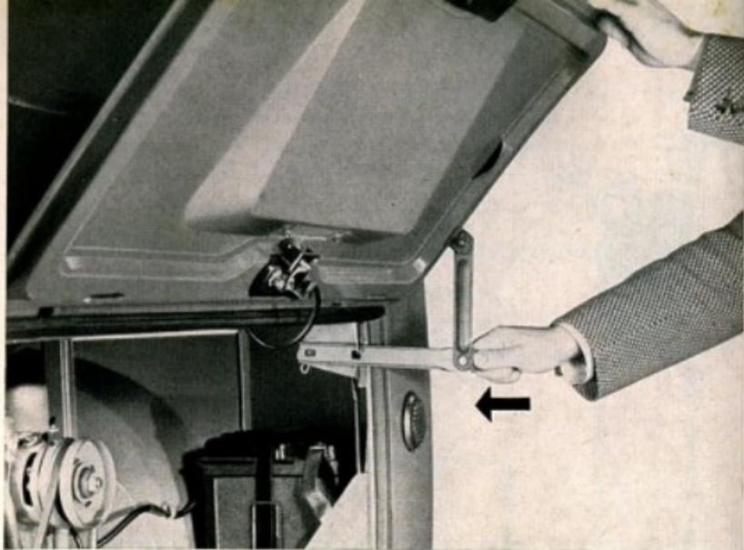
The engine compartment lid is opened by means of the square key delivered with the vehicle. The lid can be lowered by pressing against the horizontal bar of the check mechanism.
