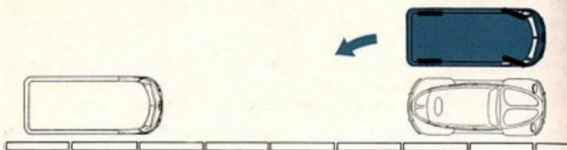
When the front bumper of your Transporter is even with the rear bumper of the car ahead of you, turn the steering wheel fully to the left, and back up further toward the curb.
