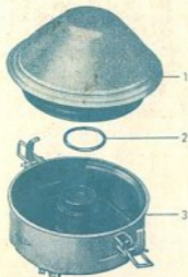
1-Filter element, 2-Gasket, 3-Oil reservoir
