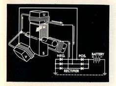
The circuit is completed through the battery to ground, through one of the negative diodes and through winding W which is negative at that moment, back to the common point of the stator windings.
