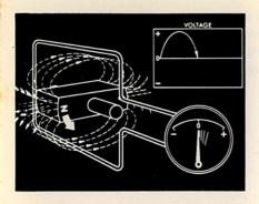
As the rotor reaches a 90° angle to the loop, there is no induction, and thus no pulse.
