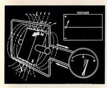
In an alternator, electrical current is produced by a magnetic field moving past a conductor and inducing voltage in this conducting loop.
