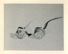
As you can see, positive and negative diodes look the same but internally each is constructed the reverse of the other. It is very important not to interchange the two types, when making repairs.
