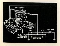
The magnetic field is created by a field or exiter winding on the rotor which carries a small amount of direct current.
