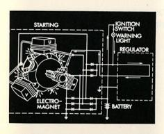
To begin with, exiter current is supplied by the battery, through the ignition switch, charging warning light and the regulator, so without some slight charge in a battery the alternator's magnetism cannot be set up.
