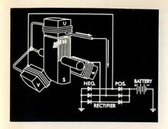
... through the positive output diode to the positive battery connection.
