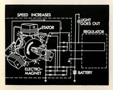
As the alternator RPM increases, the warning light goes out and the output of the stator windings supplies current to the field winding.
