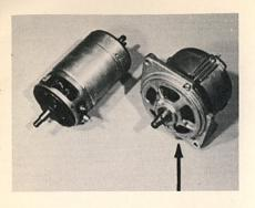
The Alternator or A.C. generator makes alternating current which must be rectified to direct current before storage in the battery.
