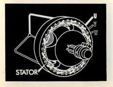
The stator is actually a slotted ring. The phase windings are distributed in sequence in the slots.
