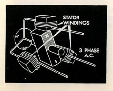
The Bosch alternator has 3 windings spaced 120° apart. Together they are called the stator and produce three phase alternating current.
