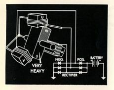
So far, we have shown the magnetic field of a rotating magnet inducing voltage in the 3 coils, but a permanent magnet large enough to create the magnetic field needed would have to be very heavy, and it would be difficult to control alternator output.
