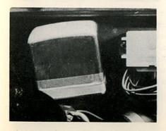
The voltage regulator is a simple switching device which is sealed and requires no adjustments.
