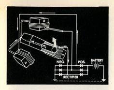
The rotor continues to turn and the positive wave pulse from winding W follows this path, while the circuit is completed through V.
