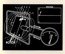
The magnet which produces the magnetic field is called the rotor.
