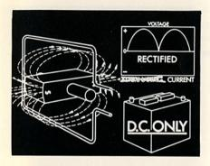
Therefore, the alternating current or A.C. from the alternator must be rectified or changed to direct current, or D.C.
