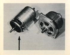
The D.C. Generator, as its name implies, makes direct current and supplies it to the automobile's electrical system and to the battery.
