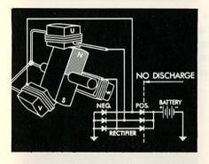
There is another important function of the rectifier diodes. They prevent the battery from being discharged through the alternator windings.
