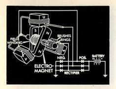
The current is provided through two carbon brushes and slip rings on the rotor shaft.
