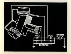
The three phase windings of the alternator are connected to three conductors which carry two diodes each.
