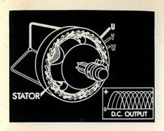
This arrangement greatly increases the output of positive pulses per revolution.
