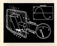
As the south pole continues to move away from the loop, voltage gradually drops off until it reaches zero, and the north pole again takes over.
