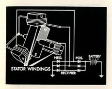
Let's see how current flows from the stator windings to the battery. The three stator windings, which we have labeled U-V and W, are joined in the center. As the rotor turns and its magnetic lines of force cut across each stator winding in turn, electrical pulses are induced in the stator windings.
