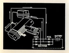
... and its pulse follows a similar course through a positive diode to the battery, and to ground then through the negative diode corresponding to the winding that completes the circuit.
