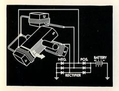
As the rotor continues to turn, winding U changes polarity due to the changing magnetic fields, and winding V becomes positive and shows up as a positive pulse on the wave form . . .
