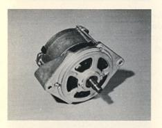
An Alternator is used on the Volkswagen 411 because it can be a more efficient source of electricity.
