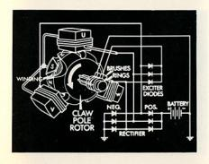
The Bosch alternator uses a claw pole rotor. The annular or ring shaped winding is surrounded by two sets of iron claws which present North and South magnetic poles to the stator in rapid succession.
