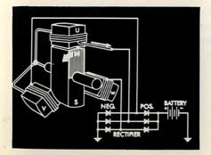
Shown here is the pulse leaving winding U, going . . .
