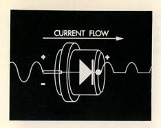
Alternating current fed through a positive diode passes only the positive half of the wave.
