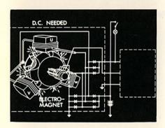
As you know, the rotor is an electromagnet. Direct current is needed to exite the rotor so it will act as an electromagnet.
