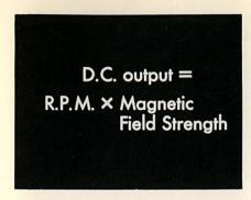
In the Volkswagen, alternator output is controlled by regulating the strength of the rotor's magnetic field.
