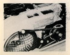
The Alternator, similar to the generator, is driven by a V-belt and is cooled by the engine fan.
