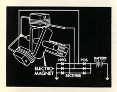
Therefore, an electromagnet is used for the rotor.
