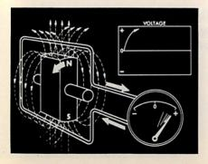
When the north pole of the magnet passes the upper loop, a positive pulse is induced in the conductor.
