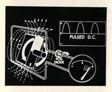
So if we place a positive diode in the upper loop of our alternator, only the positive half of the wave will get through, resulting in pulsed direct current.
