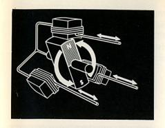
The north and south poles of the magnet pass each of the three windings in turn, inducing voltage in each coil as they pass.
