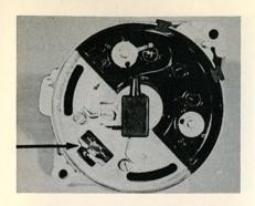
The regulator senses the battery voltage at D+/61 of the regulator terminal of the alternator.
