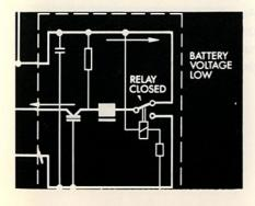
For example, if the battery voltage is low, the relay will remain closed allowing full current to flow to the field coil. The alternator will put out its maximum.
