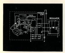
And when voltage is low, it allows current to flow to the field winding of the rotor, thus inducing more voltage in the stator windings.
