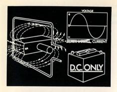
This alternating current cannot be used by the automobile system because only direct current can be stored in the battery.
