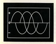
... we have three overlapping waves equally spaced.
