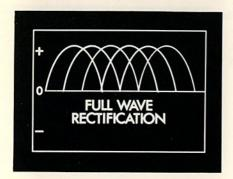
Thus, the direct current leaving the positive diodes now carries not only the positive portions of our A.C. wave, but also the negative portions which now appear as positive pulses. This is full wave rectification.
