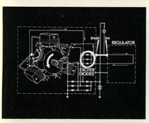
Their positive poles meet at terminal D+/61 of the alternator. The same terminal which the regulator is connected to.
