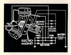
The brushes get current from three exiter diodes which rectify the alternating current generated in the stator windings.
