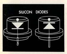
Conversion from A.C. to D.C. or rectification is done by Silicon diodes.
