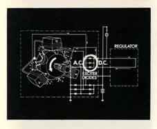
The exiter diodes rectify the alternating current generated in the stator windings for the field winding.
