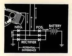
When a pulse of current arrives at the rectifier circuit, it produces a potential difference between the negative and positive diodes whether the pulse itself is plus or minus.
