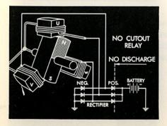
Therefore, a cut-out or reverse current relay, which is necessary for D.C. generators, is not needed for alternators.
