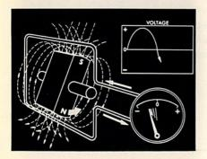
As the south pole approaches the upper loop, the pulse continues to build on the negative side. It reaches its maximum when the pole is closest to the loop.
