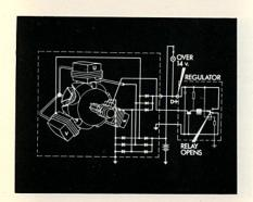
When the regulator senses over 14 volts in the battery, a relay opens, cutting off current to the field winding.
