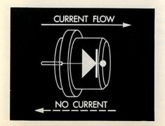
A diode is a semi-conductor device that allows current to flow in only one direction. It is like a one-way valve.
