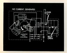
Of course, when the field winding on the rotor gets no direct current, its magnetic field collapses and without magnetism it can no longer induce current in the stator windings. The alternator stops generating current even though the rotor continues to turn.
