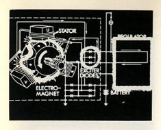
This current is passed through the exiter diodes and through the regulator, to the positive pole of the rotor.
