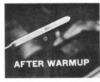
In most cases you will find that the fluid level is now between the two marks, as it should be. If it is not at the proper level --that is between the two marks--add some more ATF. Remember, the difference between the two marks is only about 8/10 of a pint. Be careful not to overfill!
