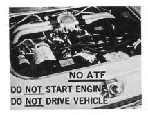
One special caution-never start the engine whenever the pan is off, or whenever there isn't any ATF in the transmission.
