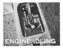
As with the Automatic Stickshift, you begin by checking the ATF level; only this time there's a significant difference. The fluid is checked with the *engine running* at idle speed, with the selector lever in "neutral". The fluid should be warm ...not cold, not really hot.
