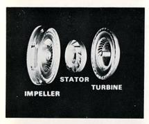
Located between the impeller and turbine is the stator a small wheel-like component. Its job is to redirect the fluid from the turbine back to the impeller. The secret of multiplying torque lies in the design of the stator.
