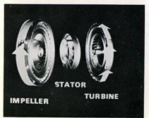
During acceleration, when more torque multiplication is needed, the impeller is driven faster than the turbine.
