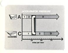
"Kickdown" is used primarily for rapid acceleration at moderate speeds. For example, if you engage "Kickdown" below a speed of approx. 53 mph the transmission will automatically down shift ... until the pressure on the accelerator pedal is released, or a speed of approximately 55 mph is reached ... then, it will upshift again automatically.
