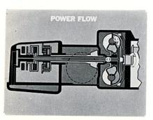
Now we examine the actual power flow through the transmission.... The engine's crankshaft drives the impeller, number 1, which drives the turbine, number 2, as described earlier. The turbine is attached by splines to the transmission input or turbine shaft, number 3.
