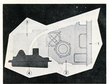
Now let's get into the major components of the transmission itself. At the rear, number 1, is the torque converter ... number 2, the final drive assembly ... number 3, planetary gear and clutches and number 4 ... the hydraulic shift controls.
