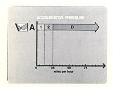
Throttle position is a control factor for shifting. Therefore, a light gradual pressure on the accelerator will cause the transmission to upshift from 1st, to 2nd and then to 3rd at approx. 15 miles per hour.
