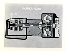
Power is transmitted by the turbine shaft, number 3, to the forward clutch, number 4, which is engaged in all forward driving ranges. The direct and reverse clutch number 5 is engaged only in direct drive (third gear) or reverse.
