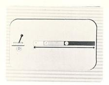
In "D" or drive the transmission automatically shifts into first gear and moves forward, then into second, and as speed increases, into third.
