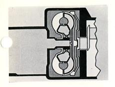
A torque converter serves two functions—first it acts as a hydraulic clutch that transmits engine power or torque to the transmission. Second, it steps up, or multiplies engine torque under certain operating conditions.
