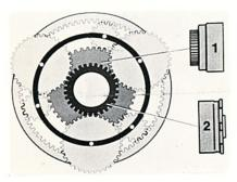
The Volkswagen planetary gear is driven by two clutches ... number 1—the forward clutch and number 2—the direct and reverse clutch.
