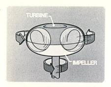
Adding a turbine on top would cause the fluid to follow a circular path and return to the impeller.
