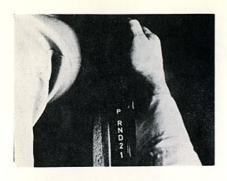
As you have seen, shifting of the automatic transmission is directly controlled by the driver through shift lever positions and accelerator pedal pressure.
