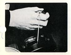
Slamming the shift lever into reverse when the vehicle is moving forward will result in damage to the transmission. So to avoid mishaps, the driver must lift the lever to select reverse or park as illustrated here.
