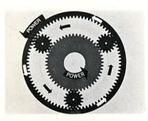
If any two members of the planetary and driven at the same time they will lock and there will be no increase in torque. The entire planetary unit would revolve and direct drive would result as in high gear range.
