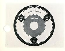
A simple planetary consists of a sun gear (Red) around which planet gears (Blue) rotate. The planet gears run on a planet carrier (Yellow) and are in constant mesh with the ring gear (Brown).
