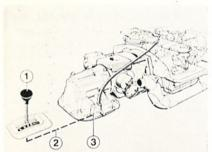
Let's begin where the driver begins—with the selector lever—shown here as number one. Number two is the linkage that connects the selector lever with the trans — mission lever.
