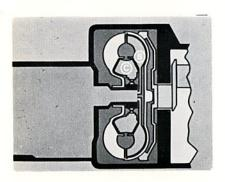
The turbine (B) which drives the transmission, and the stator (C) which is used to multiply torque.
