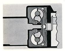
The torque converter is composed of the impeller (A) which is connected to and driven by the engine.
