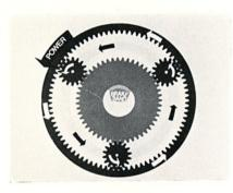
If, however, the Sun Gear is held and the ring gear is driven, the planets would "walk around" the sun gear, causing the planet carrier to turn within the ring gear. Again, resulting in an increase in torque, but not as great as before. This would be similar to an intermediate range on an automatic transmission.
