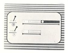
If, the 2nd gear position is selected, the transmission will start off in 1st gear, then shift automatically into 2nd and remain there.
