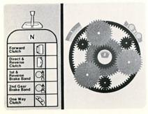
This diagram of the planetary with its three holding devices . . . Number 1—First and reverse brake band
