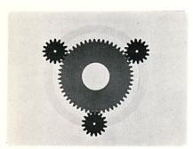
that are connected by a planet carrier which transmits all power to the differential.
