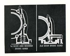
In addition, two brake bands, that act as hydraulically operated holding devices, are used for shifting. The 1st and reverse brake band, which holds the ring gear, is applied whenever the shift lever is in the 1st or reverse gear position. The 2nd gear brake band, similar in design, is applied whenever second gear is engaged.
