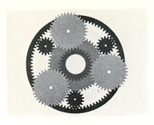
meshes with large planet gears that are also supported by the planet carrier.
