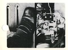
The "Kickdown" switch is located under the gas pedal on Types 2 and 4 and on the throttle lever of Type 3's. In either case, it must be correctly adjusted so it operates neither too early nor late when the accelerator is fully depressed.
