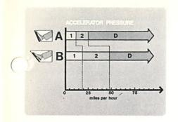
Heavier pressure on the accelerator delays shifting, uses more fuel but increases acceleration by allowing the engine to rev much higher in each gear range.
