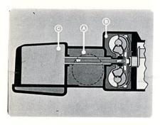
Let's look at the complete unit . . . a hollow turbine shaft (A) connects the torque converter (B) to the transmission assembly (C). ATF flows between the torque converter and the transmission through the hollow turbine shaft.
