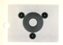
A large sun gear meshes with small planet gears
