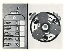
The main object of selector lever position 1 is to use full engine braking power. When lever position one is selected the forward clutch is applied as before but the first & reverse brake band is also applied. This locks the ring gear, keeping it from turning in any direction, and allows the car to decelerate against engine compression.
