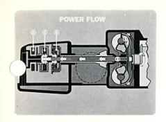
From the clutches the power passes into the planetary gear set (number 6) which produces the three forward and one reverse gear ratios.
