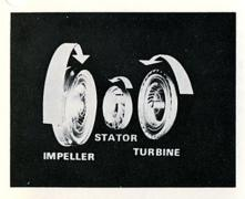
As the turbine turns faster and faster, it eventually approaches the speed of the impeller and then torque multiplication falls off.
