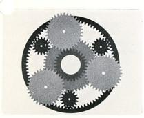
The planetary gearset is the heart of any automatic transmission. It is an assembly of constant mesh gears, that can change ratio depending on which gears are held and which gears are driven. The double planetary in the Volkswagen transmission is very compact considering that it can develop 3 forward and one reverse gear ratio.
