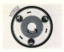
If the ring gear is held and power is applied to the sun gear, the planets would be forced to rotate and "walk around" the ring gear. The planet carrier would also revolve but at a slower speed than the sun gear and the result would be increased torque similar to low range on an aut matic transmission.
