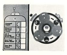
When Reverse is selected, the direct & reverse clutch is engaged driving the small sun gear. The first and reverse brake band is also applied locking the ring gear and the result is Reverse.
