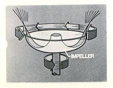
If the impeller were in this position . . . filled with fluid, then spun centrifugal force would cause the fluid to spin out as shown here.
