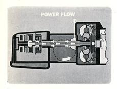
The planetary gear set is coupled directly to the pinion shaft, number 7, which drives the differential and the road wheels.
