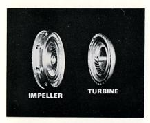
In an actual torque converter, both the impeller and turbine have vanes. Fluid which is guided by the impeller vanes actually drives the turbine by striking its vanes under the pressure of centrifugal force.
