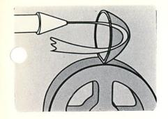
To understand torque multiplication, think of the impeller as a nozzle spraying fluid into this cup on the turbine wheel. Due to its shape the fluid from the impeller is directed out of the turbine cup and a lot of it's force is wasted.
