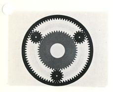
The small planet gears are also in mesh with the ring gear.
