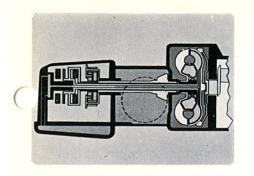
We have also seen how this torque reaches the VW planetary gearset and how 1st, 2nd, 3rd and Reverse are developed through the use of combinations of clutches and brake bands.
