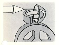
The stator is like this curved piece, it redirects the otherwise wasted fluid back into the cup so that the remaining force of the fluid is added to the force that was transmitted when the fluid first hit the cup.
