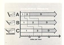
Full accelerator pressure, pressing the accelerator all the way down to the floor, further delays shifting by engaging "The Kickdown" letting you accelerate even faster.
