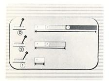
And for maximum braking effect on steep down grades, the 1st gear position can be selected, however 1st gear will remain engaged until manually shifted into 2nd or the Drive gear range.
