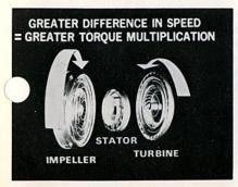
Torque multiplication is only possible when there is a difference in speed between the impeller and turbine. The greater the difference in speed, the greater the torque multiplication.
