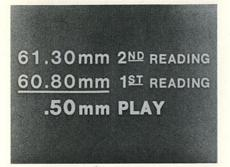
The .50mm difference between these two readings is the ball joint play.
