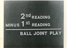
From here on it is the same, compare the first reading with the second, and the difference is the ball joint play.
