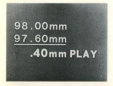
Once again, the first reading is subtracted from the second, and the resulting figure is the play of the ball joint.
