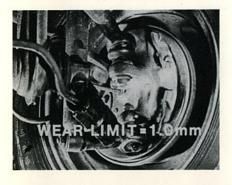
On Type 1 vehicles the wear limit for lower ball joints is 1.0mm.
