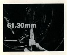
Check the caliper reading again. It's the difference between the 1st and 2nd reading that we are interested in.
