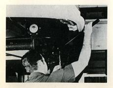
... then pull down on the lever handle. This raises the lower torsion arm so that the play can be read.
