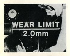
The wear limit for Type 2 lower ball joints is 2.0mm. If the play had exceeded this amount, the ball joint would have had to be replaced.
