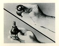
Should the seals or plugs become broken or cracked, dust, dirt, or water can enter the ball joint and damage it. Cracked or broken seals or plugs must be replaced.
