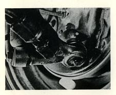
Therefore, the amount of play in each joint must be checked, to make sure they are within "wear limits".
