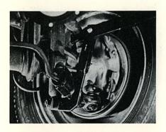
Here's how these tools are used on Type 1 vehicles. First, insert the checking lever between the upper and lower torsion arms as shown here.
