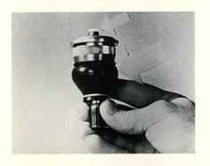
Finally, another important point to remember when you are checking ball joints — you should always check the dust seals and the plastic plugs for cracks or leaks.
