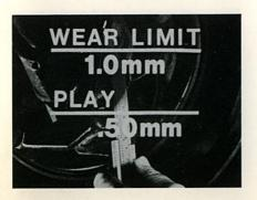
Since this ball joint is well within wear limits, no replacement is needed.
