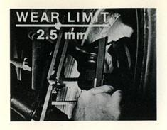
The wear limit for the upper ball joint is 2.5mm.
