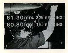
It is substracted from the second reading, 61.30mm, taken from the caliper after pulling down on the checking lever.
