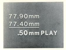
Subtract the first reading from the second, and the difference is the ball joint play.
