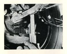
One jaw of the caliper is placed on the lower section of the steering knuckle, and the other jaw on the lower torsion arm.
