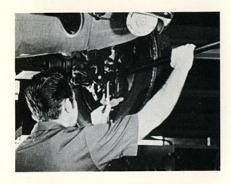
Position the lever over the torsion arms, and place the caliper on the lower ball joint.
