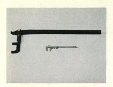
A vernier caliper and the special ball joint checking lever are used to accurately determine the amount of ball joint play.
