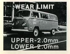
The wear limit for the Type 2 upper and lower ball joint is the same.
