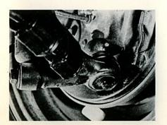
Ball joints serve as pivots permitting easy steering and up-and-down movement of the stub axle, as the vehicle moves over the road.
