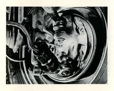
The front wheel ball joints are checked during diagnosis and maintenance and from a saftey point of view, this is an extremely important check.
