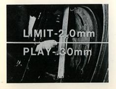
Since this ball joint is also within wear limits, no replacement is needed.
