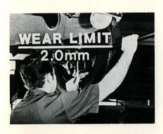
The wear limit for a Type 3 lower ball joint is 2.0mm.
