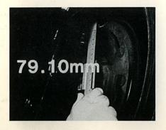
The procedure is the same: take a reading when the caliper is first placed on the ball joint.
