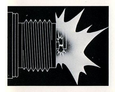
The object of the system is to get the battery to furnish enough voltage to make a spark jump across the gap of the spark plug electrodes.
