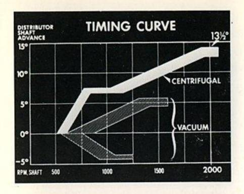
And at 2,000 RPM, rotation should be at its maximum 13 and a half degrees.
