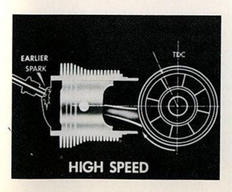
At high speed, it is necessary to deliver the spark to the combustion chamber earlier to give the mixture ample time to burn and deliver its power to the piston.
