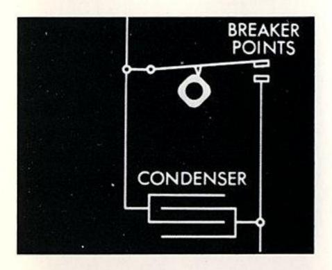
One very important component in creating the high voltage current which fires the fuel-air mixture is the condenser. The condenser is connected across the ignition breaker points. It has two functions.
