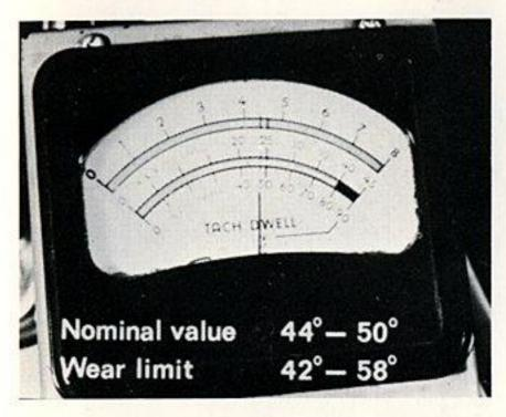
If the points are new, the reading should be between 44 and 50 degrees. Old contacts should not be adjusted as long as the reading is within the wear limit, 42 to 58 degrees.
