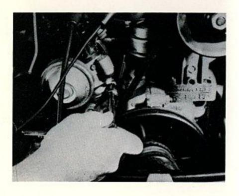
Slightly loosen the nut holding the distributor. Now, start the engine . . .
