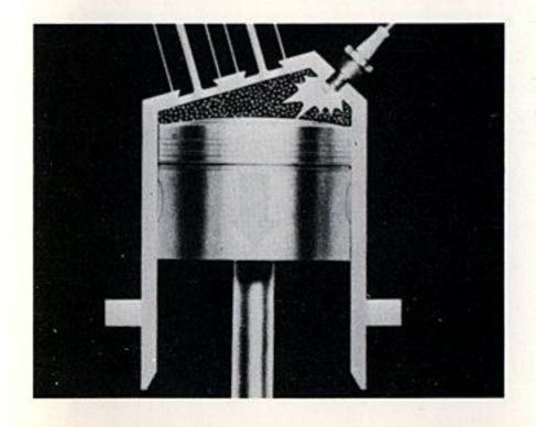
Then comes the spark and the power stroke as the expanding gases of the burning fuel force the piston down.
