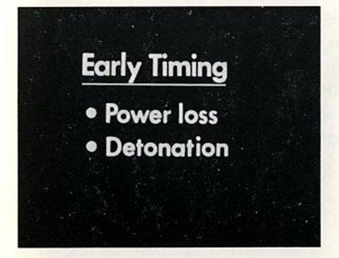
We can summarize incorrect timing in two broad categories. Early timing will mean loss of power and/or detonation, because the engine is fighting itself.
