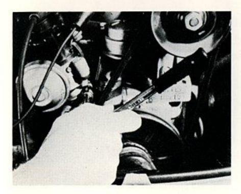
Tighten the nut securing the distributor, and recheck with the timing light. If it has not moved and the idle speed is still correct, the basic timing is completed.
