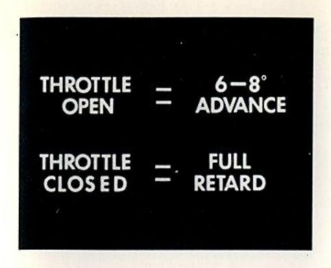
The result is — as soon as the throttle is opened, the advance jumps ahead 6 to 8 degrees; and when it is closed, the spark is quickly and fully retarded.
