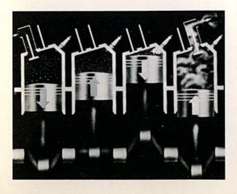
As we know, in the 4 stroke cycle engine, each cylinder fires every second revolution of the crankshaft.
