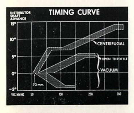
With the throttle open, the vacuum advance starts to operate at 70mm of mercury.
