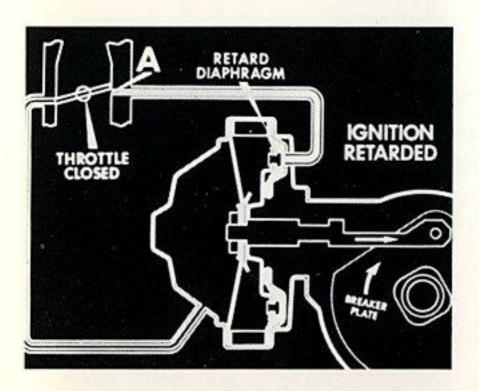
When the throttle is closed, a vacuum at tube A acts on the retard diaphragm which moves the breaker plate to retard ignition.
