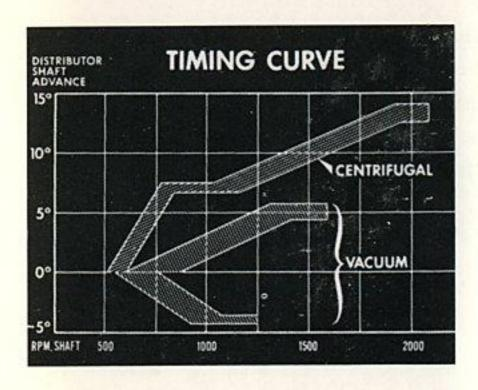
Note that RPM and degrees of advance are expressed in distributor shaft rotation and not crankshaft RPM, which would be twice as much.
