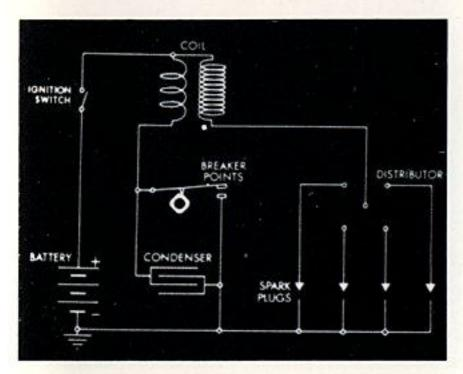
Here is an ignition circuit with the parts indicated. They are: the battery, ignition switch, ignition coil, breaker points, condenser, distributor and spark plugs.
