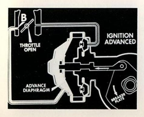
When the throttle is partly opened, it uncovers tube B, causing a vacuum which acts on the advance diaphragm, moving the breaker plate to advance ignition.
