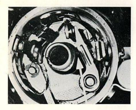
To adjust the points, turn over the engine by hand until the rubbing block is on the highest point of the cam.
