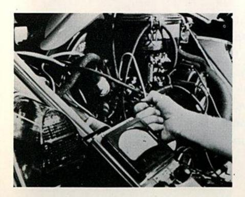
To check, attach a dwell meter between the distributor side of the coil and ground, according to the Workshop Manual or manufacturer's specifications.
