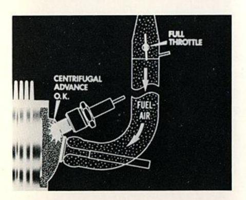
The centrifugal advance takes care of conditions of full throttle at high speed and acceleration at medium speed, but there are other situations requiring spark advance that it can't cope with.
