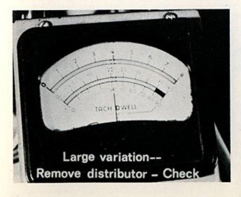
A large variation in the dwell angle indicates distributor shaft wear and the distributor should be removed and checked. If the reading is within limits, no adjustment is necessary.
