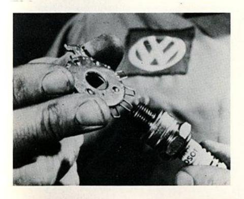
If they are in good condition, clean them and adjust the electrode gap; if they are badly worn or damaged . . .
