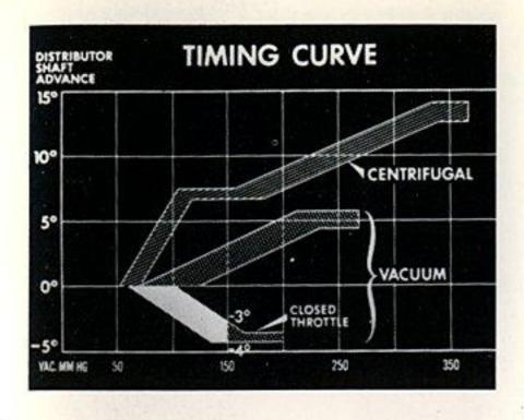
With the throttle closed, the distributor shaft is retarded between -3 and 4 degrees when the vacuum reaches 150mm of mercury.
