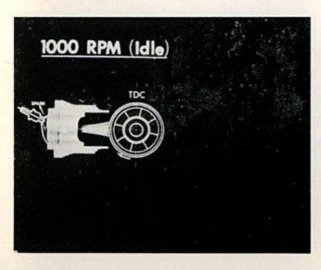
At 1,000 RPM, there is enough time during the power stroke to burn the fuel completely.
