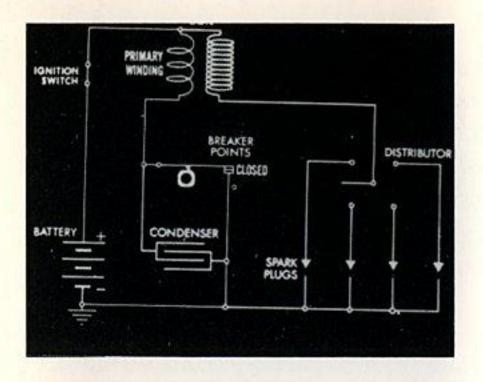
The voltage is increased by the coil working with the breaker points. As the ignition switch is turned on, current flows from the battery, through the primary winding of the coil, and through the breaker points when they are closed.
