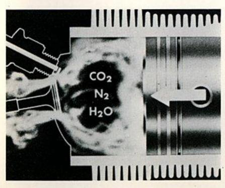
When the power stroke is finished, ideally the fuel will be completely burned, and the by-products coming out during the exhaust stroke will be Carbon Dioxide, nitrogen and water vapor. Our objective is to come as close to this ideal as possible.
