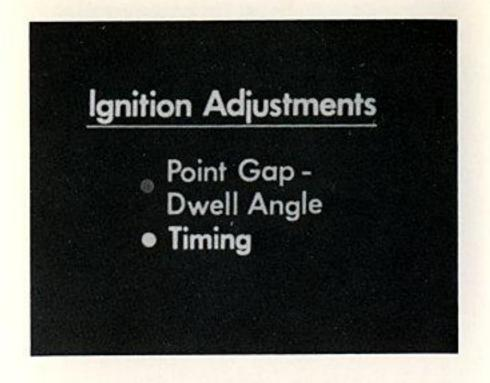
Whenever the dwell angle is adjusted or breaker points changed, engine timing must always be adjusted.
