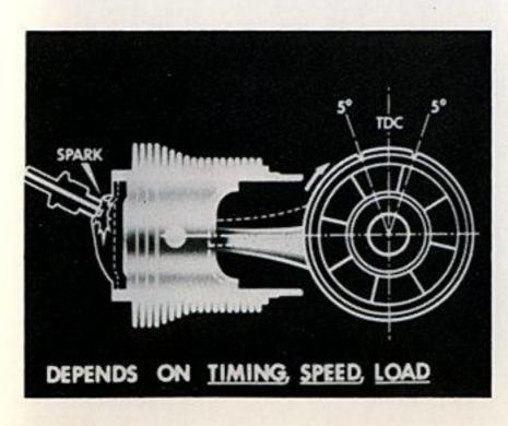
Where the piston is in relation to Top Dead Center when the spark occurs, depends on how the timing is set and how the automatic advance-retard controls work in response to engine speed and load.
