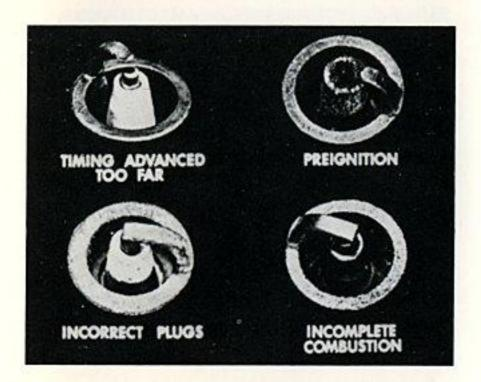
These plugs show only four of the many problems that can be diagnosed by careful inspection. Ignition timing advanced too far, Pre-ignition or detonation, fouling caused by incorrect spark plugs, incomplete combustion.
