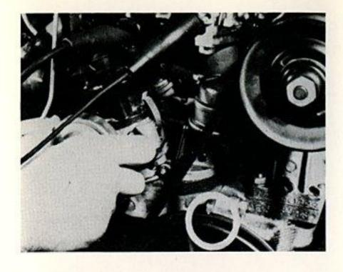
If not, twist the distributor until the notch lines up. Your spark is now firing at factory specifications.
