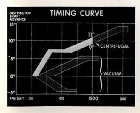
At 1,500 RPM, rotation should be between 9 and 11 degrees.
