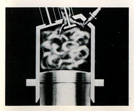
After the fuel is burned, the piston goes up again in the exhaust stroke forcing the combustion by-products out of the now open exhaust valve.
