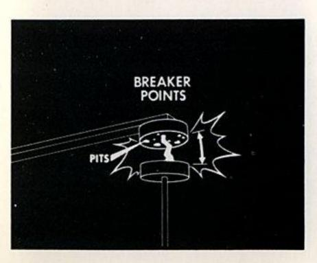
First, as the breaker points open, they tend to arc. This may cause the breaker points to pit or burn.
