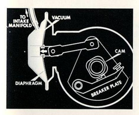
When the diaphragm moves out against spring tension, the breaker plate moves with it and carries the breaker points along so that the cam, as it rotates, closes and opens the breaker points earlier in the cycle.
