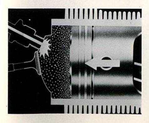
For example, let's say we get a spark when the piston is only three quarters up and compression rate is at its maximum.
