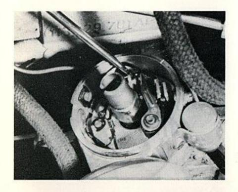
After loosening the retaining screw that secures the point assembly, adjust the dwell angle by twisting a screwdriver between the two small pins on the breaker plate and a slot on the point assembly base,
