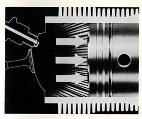
The burning process causes a rapid expansion in the gases, causing a pressure on the piston and driving it down.
