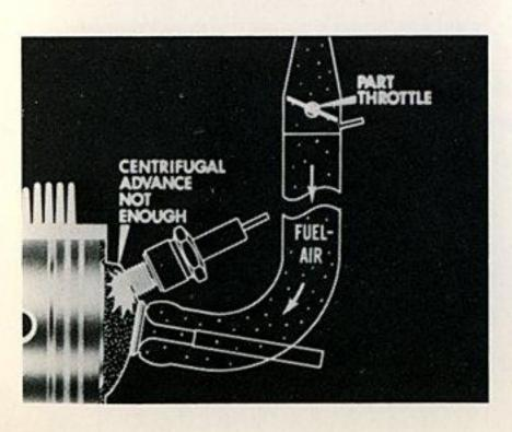
At part throttle, where maximum power is not being demanded of the engine, compression pressures are lower, the rate of combustion is slower, but it is still necessary to advance the ignition timing to obtain satisfactory burning of the fuel-air mixture.
