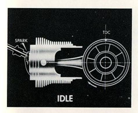
As we know, at idle speed the spark is adjusted to occur at approximately the point where the piston reaches Top Dead Center. The exact point will vary a few degrees, depending on model and latest factory specifications.
