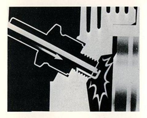
The current then flows down the center of the plug, jumps the gap between the electrodes to produce a hot spark and is grounded to the engine block.
