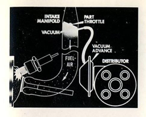
In this situation, the engine speed is too low to throw the weights out far enough, so the vacuum advance helps out. It works like this. Under part throttle a vacuum develops in the intake manifold.
