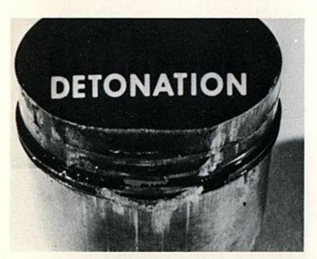
This is what can happen. The piston head has literally disintegrated due to persistant detonation.
