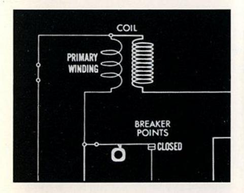
With the points closed, the ignition circuit is completed and a . . .
