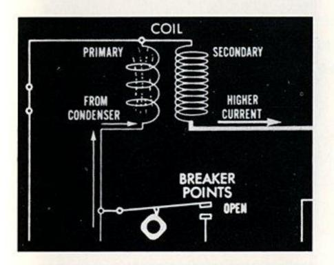
Second. After the points have separated and there is no longer any danger of an arc, the current that has been stored in the condenser flows back into the coil, opposing the primary magnetic field which is already collapsing. The faster the field changes, the higher will be the current induced in the secondary.
