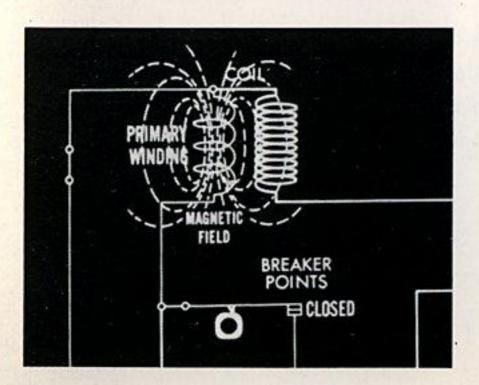
... magnetic field is set up in the primary winding of the coil. Any change in this field will induce a high voltage current in the secondary winding, because it has many more turns than the primary.
