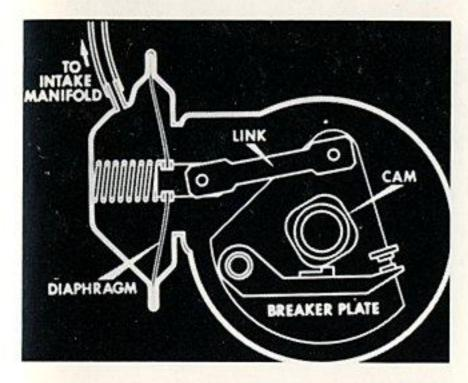
The vacuum acts on a diaphragm which is linked to the breaker plate.
