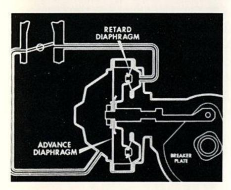
Briefly, there is a separate diaphragm and vacuum chamber for retard position that works opposite to the advance diaphragm.
