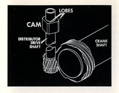
The cam has 4 lobes, one for each cylinder. It is at the end of the distributor drive shaft which in turn is driven by the engine crankshaft.
