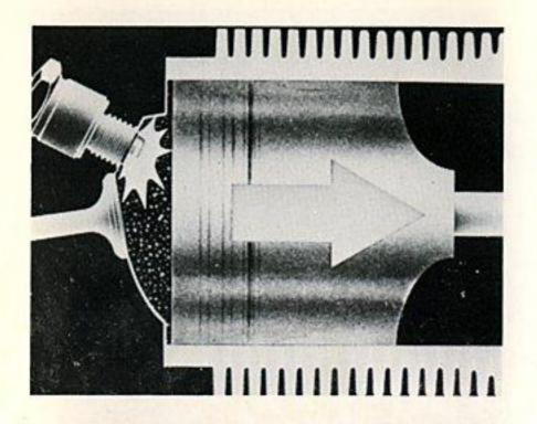
It is obvious that the spark should occur at exactly the right time to ignite the fuel-air mixture so that it burns as efficiently as possible. But why should this timing vary?
