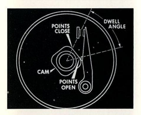
The first adjustment is to set the dwell angle of the breaker points. Dwell angle simply means the number of degrees of distributor cam rotation from the instant the breaker points close until they open again.
