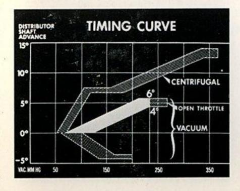
At 230mm, the vacuum advance reaches its maximum and no increase in the vacuum will cause this system to advance the spark any further.
