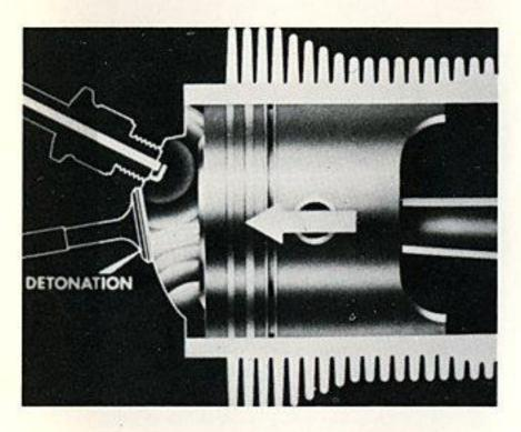
The two flame fronts meet and the resulting detonation causes a noisy hammering pressure on the piston and stresses on other engine parts.
