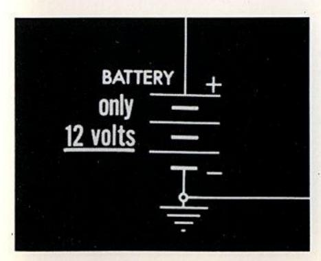
But a modern automobile battery puts out only 12 volts, far too little to cause this to happen, so we have to find a way to increase the voltage many times.
