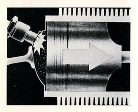
The job of the ignition system is to assure that sufficient voltage is delivered to the spark plug of the correct cylinder at the exact instant that the piston is in position to make the most efficient use of the burning fuel-air mixture.
