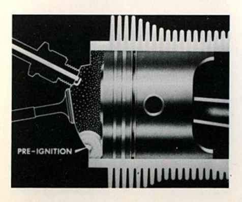
The effect of pre-ignition is very similar to detonation. The main difference is that the spark plug fires after the false ignition instead of before.
