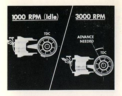
But the time available from Top Dead Center at, say, 3,000 RPM is two-thirds less than at 1,000 RPM. Therefore, in order to have maximum pressure at the correct time at higher RPM, it's necessary to "light the fire" earlier — or advance the ignition timing.
