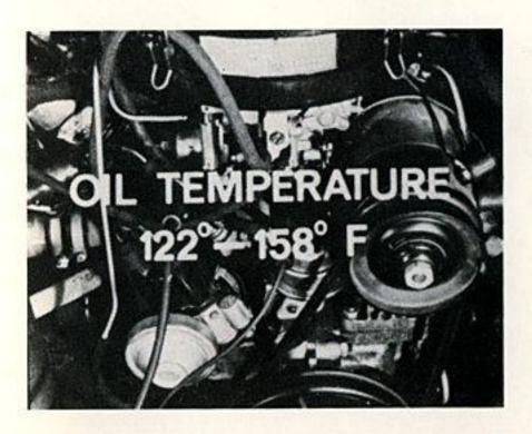
The engine must always be at normal operating temperature, between 122 and 158 degrees F. Otherwise, tolerances will be off, and any adjustment you make will be inaccurate.
