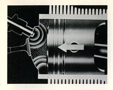
This pressure produces heat which, added to the heat of the burning fuel, causes a portion of the fuel charge to ignite spontaneously.
