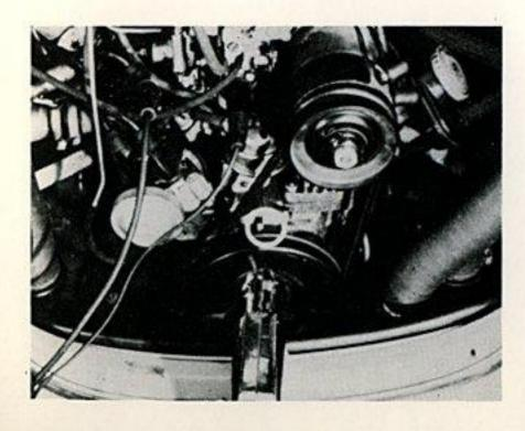
Now, aim the timing light at the split in the crankcase and observe whether the notch is in the proper place. If it is, timing is good.
