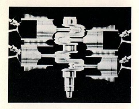
Thus, in a Volkswagen, 2 cylinders fire for every crankshaft revolution, and all four cylinders fire every two revolutions.
