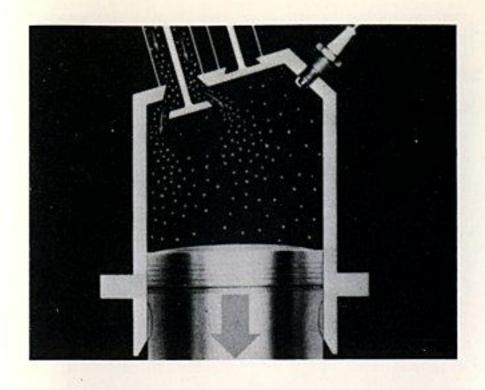
On the intake stroke, the piston goes down and draws in the fuel-air mixture.
