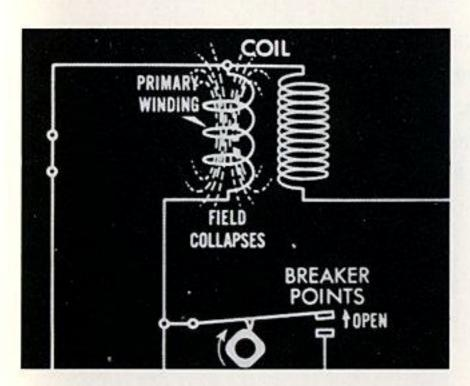
When the points open, current stops flowing through the primary winding, and the magnetic field suddenly collapses.
