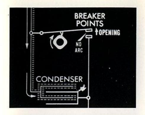
The condenser provides a place for the current to go during the first instant that the breaker points separate, so that it doesn't arc across the opening points.
