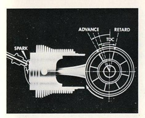
Other combinations of load and speed require different ignition advance settings, and the engine must be capable of adapting to these requirements.
