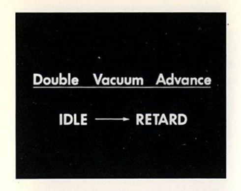
Its purpose is to assure that the spark will be fully retarded when the engine is idling, assuring fullest combustion of the fuel and, therefore, minimum exhaust emissions.
