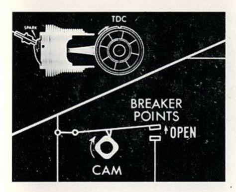
It is so linked with the crankshaft that each time a piston reaches approximately Top Dead Center of the compression stroke, one of the cam lobes opens the ignition points.
