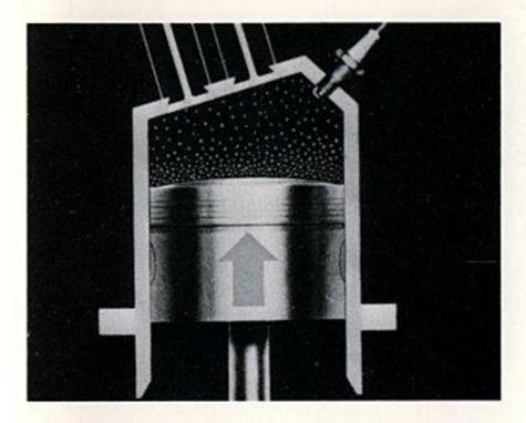
On the compression stroke, the piston goes up with both valves closed, and the fuel mixture is compressed.
