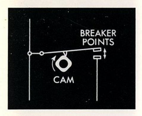
The points are opened and closed by a cam which revolves at half crankshaft speed as the engine is turned over.
