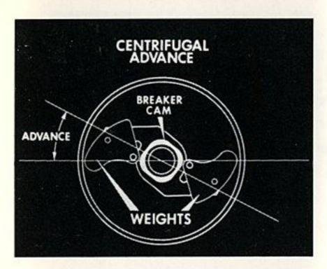
This movement is transmitted to the breaker cam and causes it to advance or move ahead with respect to the distributor shaft. The ignition timing consequently varies from no advance at low speed to full advance at high speed when the weights have reached the outer limits of their travel.
