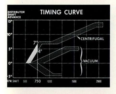
At 750 RPM, the distributor shaft should be advanced between 4 and 7 degrees due to centrifugal action.
