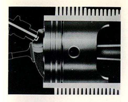
Combustion sweeps evenly across the confined area containing the fuel/air mixture.
