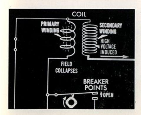
The magnetic field collapses inwards; as it collapses, it induces a high voltage current in the secondary windings, because there are many more turns in the secondary.
