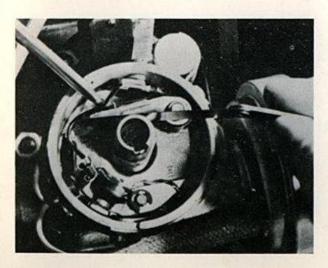
and setting the point gap to 16 thousands of an inch or .4 tenths of a mm. Tighten the retaining screw and again check the dwell angle with the meter.
