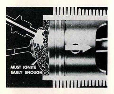
The time taken to develop maximum pressure from a specific fuel-air charge remains constant. So, we must ignite the mixture early enough to assure that as it burns and expands, it develops its maximum pressure at the point in its down stroke where the designer calculates its maximum efficiency to be.
