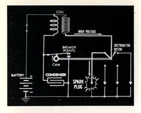
The high voltage, as much as 23,000 volts, now goes to the distributor rotor which is keyed to the breaker cam so that they operate in synchronization. At the same time the breaker points are open, the rotor is in contact with one of the four terminals connected to a spark plug.
