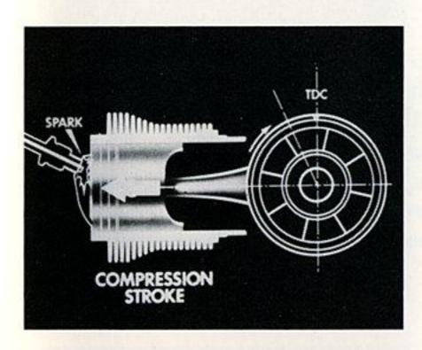
The spark should jump the gap between spark plug electrodes when the appropriate piston is at its firing point in the compression stroke.
