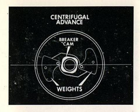
The centrifugal advance does this by two weights that throw out against spring tension as engine speed increases.
