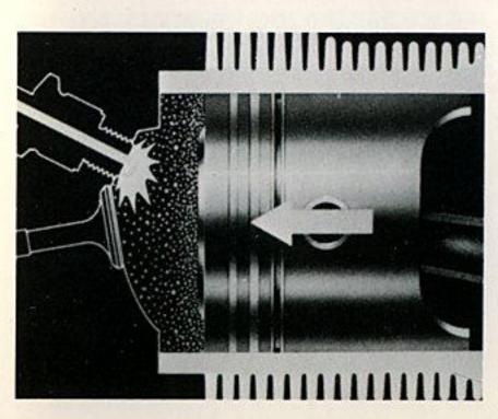
As the piston arrives at or nears the top of its compression stroke, the spark occurs and begins to burn the compressed fuel.
