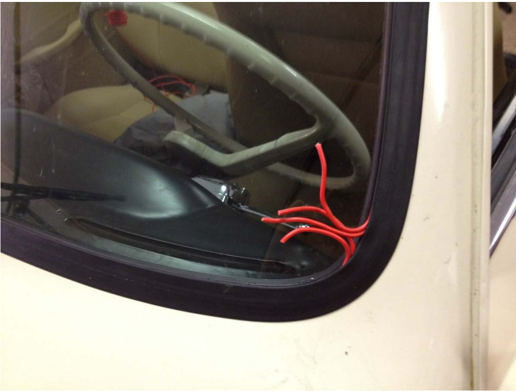
Sharpest corner with wires all in.
