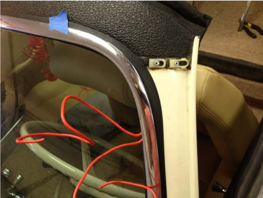
Working up the side. See how far the trim needs to be pushed into the molding.
