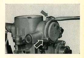
11/42 Here is a ceramic plate with a damaged center boss. The bi-metal spring can move out of its central position and this affects the opening and closing of the choke valve. In this case a new part has to be installed. At the outer edge of the ceramic plate is a copper ring which provides the ground connection between the cable terminal and the carburetor body. This ring is essential to the trouble-free functioning of the automatic choke and should be kept clean and free of grease.
