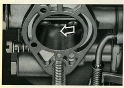
11/25 The arrow is pointing to the bypass ports which are about level with the edge of the throttle valve when it is closed. The idle port is on the left slightly more to the front. Take care that these small holes are always clean and undamaged.
