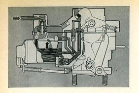
11/17 The fuel — show by the darker shade — comes from the fuel pump, enters the carburetor on the left as shown and flows through the float needle valve into the float chamber. When the fuel level is low, the float needle is in the lower position and the valve is open. The black arrow indicates the upward movement of the float.
