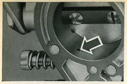
11/23 which comes out through the idle port — indicated by the arrow — below the throttle valve. On the left is the volume control screw and spring. This screw is turned to control the amount of idling mixture.
