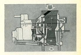
11/22 Here we have the lower part of the carburetor body. In the upper left corner you will recognise the discharge arm, to the right the float and below this the accelerator pump. The light arrow points to the pilot air drilling and the dark arrow to the pilot jet. This is where the air and fuel are combined to produce the idling mixture —
