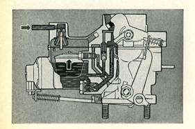
11/18 When the fuel reaches a certain level, the float closes the needle valve and the delivery of fuel stops. The small arm on the float forms a lever to increase the closing pressure. The fuel then flows through the main jet and into the other passages. The drilling on the right leads through the emulsion tube to the discharge arm. The one above it, with the ball valve, belongs to the power fuel system and the one on the left to the idling system.
