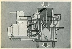
11/26 As the engine speed increases, the carburetor operation becomes normal. The fuel flows through the main jet up to the emulsion tube on the right. The fuel level is the same in the float chamber and the emulsion tube. The speed of the induced air now draws the fuel out of the discharge arm and the two combine to provide the mixture.
