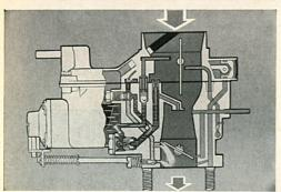
11/24 To increase the engine speed, more fuel is required. A slight pressure on the accelerator opens the throttle a little wider. The transfer from idling to normal running is taken care of by two small drillings known as by-pass ports. They are located to the left of the throttle valve and connected to the idling passage. They provide the engine with an additional supply of idling mixture.
