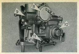
11/4 The right side shows: 8 the ceramic plate with cable connector secured to the upper part of the carburetor body by means of a retaining ring. Below it is the pilot jet. The vacuum piston works in the small cylinder 9 cast onto the side of the ceramic plate housing. The accelerator pump 10 is connected to the throttle valve shaft 11 by a rod.
