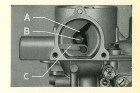
11/10 When the vacuum piston — indicated by the dark arrow on the right — slides outwards, it opens the choke valve against the tension of the bi-metal spring. A drilling in the carburetor body leads from the vacuum cylinder to below the throttle valve. The other arrow shows the position of the choke valve just before the piston reaches the outer end of its stroke. Behind the choke valve you can see the piston rod, the lever on the choke valve shaft and the bi-metal spring.
