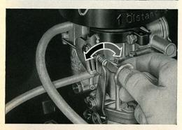
11/38 If the idle adjusting screw is turned to the right, as shown by the right-hand arrow, the speed increases. Turning to the left reduces the speed.
