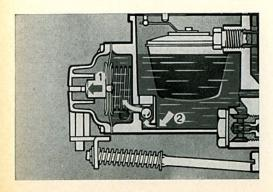
11/32 The accelerator pump works in the same way as on the 28 PCI carburetor. The pump is screwed to a housing near the float chamber. The suction stroke takes place just before the throttle valve closes as the pump spring forces the diaphragm outwards in the direction of arrow 1. This draws fuel via the ball valve into the pump chamber as shown by the arrow at 2. On the delivery stroke the fuel is pumped out of the chamber via the dark colored drilling shown below the pump spring.
