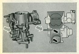
11/6 We have already mentioned the vacuum connection for the spark advance mechanism. Here you see the connection tube, indicated by the light shaded arrows. The vacuum is taken from the points shown by the black arrows in the cutaway view. The upper point is at the narrowest part of the venturi and the lower point is in the area where the throttle valve seats when closed.
