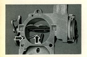
11/31 This is a picture of the upper part of the carburetor body as seen from underneath. The left arrow points to the drilling for the power fuel system which leads up to the right angled tube. The arrow in the center shows the discharge hole.
