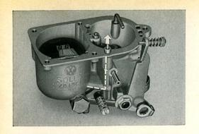
11/30 The dotted line shows the path of the fuel from the float chamber up through the carburetor housing. The ball valve is in the upper half of the vertical drilling. The carburetors for the Karmann Ghia and Transporter engines are not fitted with the ball valve because the suspended type oil bath air cleaner alters the induction conditions at the choke valve.
