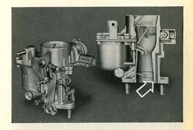
transmitted to the choke valve shaft by the piston rod and the lever. The choke opens and increases the proportion of air in the mixture so that it automatically becomes weaker.
