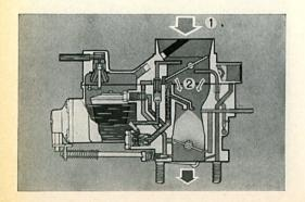
11/19 We now return to the starting procedure. The air is drawn in as shown by the arrows at 1 and 2 and accelerated below the choke valve by the venturi. This creates a depression or vacuum. The fuel flows through the main jet to the emulsion tube and is drawn out of the discharge arm by the induced air to form the mixture.
