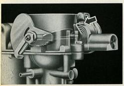
11/7 This sectional view shows parts of the automatic choke. The disc in the center is the choke valve which is mounted off center in the shaft so that the two parts are of unequal sizes. On the left is the operating lever which is fixed to the choke valve shaft and the freely pivoted fast idle cam. The lever on the right near the arrow is also fixed to the choke valve shaft. The arrow indicates the contact between this lever and the bi-metal spring which is bent to form a hook at the end.
