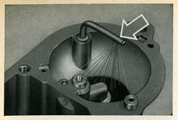
11/36 Here you see the venturi in the lower part of the carburetor with the arrow indicating the discharge tube. The size of the hole is calculated so that the fuel spray continues as long as possible and is directed straight into the mixing chamber.
