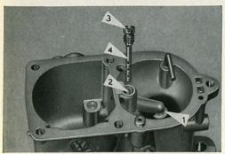
11/5 Here is the lower part of the carburetor body. On the left is the float chamber and on the right the venturi which is cast into the housing and cannot be replaced. In the center of the induction passage is the discharge arm 1 which is connected to the vertical drilling 2. The air correction jet 3 is screwed into this drilling and carries the pressed-in emulsion tube 4.
