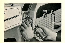
21/32 As you will know the door hinges are no longer lubricated in the factory. This is done to prevent damage being caused by drops of oil. The hinges must now be oiled. Use a thin graphite penetrating oil and clean off the superfluous oil ofterwards.
