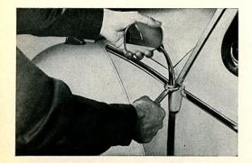
21/28 A 16 mm open-end wrench is one of the tools used during Delivery Inspections. It is required when fitting the exterior mirror. Do not use a 17 mm wrench as this will damage the chrome on the nut. We insert the mirror arm fully into the hinge pin and tighten the nut when the arm is at 90° to the axis of the car.
