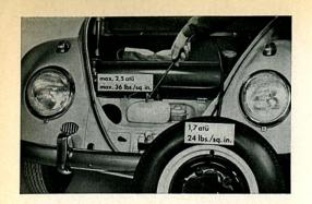
21/22 Fill the windshield washer container up to the top with clean water and pressurize it to 2.5 kg/sq. cm (36 p. s. i.). Make sure that the cap and the valve etc. are not leaking. Some dealerships fill in pure spirit in winter to prevent the washer from freezing. Now check the spare wheel pressure. It should be at least 1.7 kg/sq. cm (24 p. s. i.) or even slightly higher.
