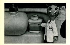
21/23 In the factory the brake reservoir is filled up to the upper edge of the mounting bracket. <sup>3</sup>/<sub>4</sub> full is sufficient. If the system requires topping up we use Genuine VW Brake Fluid or Lockhead brake fluid. After topping up we have to check the brake system for leaks later on when the car is on the hoist.
