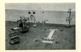
21/9 The Delivery Inspection has much in common with a Maintenance Service. The work bay is very similar to the Maintenance Service Stand: apart from the hoist, tools, various lubricants and cleansing materials etc. there should also be a tire inflator and a headlamp aiming device.
