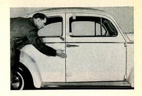
21/30 After we have convinced ourselves that the three striker plate mounting screws are tight we open and close the door a few times to check whether the door closes properly. The door must not rattle in the lock and the closing pressure must not be excessive as otherwise the door will tend to spring back when being closed.
