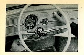
21/37 We now switch on the flashing indicators and the lights. When the flasher relay ticks the green dual arrow must light up. With the parking lights switched on the instrument panel lighting must come on. It must also be possible to regulate the panel lighting by turning the knob. When the headlights are switched on we check the dimmer switch. On high beams the blue warning light must light up.
