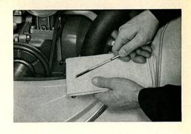
21/16 The fan belt tension can be checked by depressing the belt with the thumb. The dimension a is 1.5 cm (.6"). Everybody knows that the tension can be altered by removing or inserting spacer washers at the generator pulley. If the fan belt is damaged, it must be replaced.
