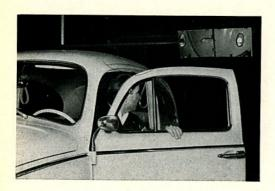
21/38 It is also important to know that all the rear lights are working correctly. With the help of a mirror as shown here it is possible to check the rear lights without the assistance of a helper.
