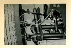
21/43 Obviously the factory pays the closest attention to ensuring that all the nuts on the steering and tie rods are correctly secured. As far as safety is concerned, double checking does no harm. The screw connections are marked in white here. Please check the brake line connections and note the position of the front brake hoses. The arrow indicates that the VW 1200 brake hoses should always be arched towards the front so that they will not rub against any part when the wheels are locked.
