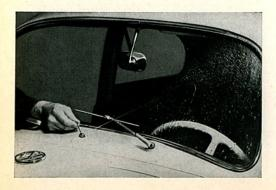
21/24 To prevent the jet of water from being blown away when driving fast, the jet should not be set too high. With the help of a pin we set the jet so that the jets of water hit the center of the windshield. We should also check whether the wiper arms are correctly adjusted and that they self-park.
