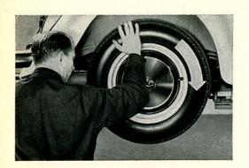
21/44 We now raise the vehicle and check the wheels by hand for even running. A slight brake drag is of no importance. If severe brake drag cannot be remedied by depressing the brake pedal heavily a few times the wheel brake has to be adjusted. If the rear wheels bind we should convince ourselves that the hand brake is fully released.
