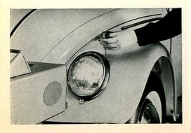
21/45 The headlamps are set with the help of optical devices on the assembly line. Since the suspension settles when the vehicle is driven on the roads, the inclination of the headlamps is consequently effected. It is, therefore, necessary that the headlamp adjustment is checked before the vehicle is handed over and corrected if necessary.
