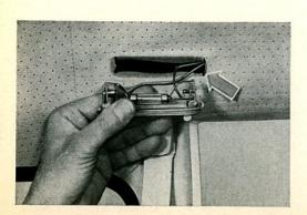
21/39 The interior light must be correctly grounded if it is to function correctly. The mounting screws provide the door contact switches with a good connection. If the interior light does not function when the switch is in the continuous lighting position we first of all check whether the spring contact on the right-hand lower edge of the light housing is perhaps insulated by the headlining. The headlining must be cut away sufficiently at the location indicated by the arrow.
