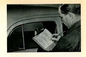
21/11 It is usual to fill up with petrol before the Delivery Inspection starts. This gives us the opportunity of carrying out an important check: checking the fuel gauge. To do this the car must be on level ground. The customer must be in a position to rely on the fact that when the needle reads R there are at least 5 liters (1.1 Imp. galls.) in the tank. If after filling in 5 liters the needle is not dead on the reserve mark, we have to set the fuel gauge.
