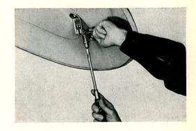
21/21 We should now carry out stocktaking under the front hood. Make sure that the spare wheel, jack, tool kit and spare fan belt are not missing. Check whether the tools are complete. Customers often complain later on that one or other of the wrenches was missing.
