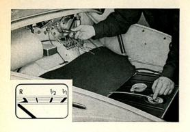
21/13 First of all we must remove the compartment lining and the tank unit cover plate. Again a helper observes the fuel gauge. We depress the float arm to the empty position, shown here as naught and turn the adjusting screw anti-clockwise until the needle clearly moves in the direction of R. We now turn the screw clockwise until the needle is positioned at the tapered end of the reserve.
