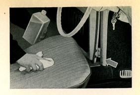
21/35 We now check the seat adjustment. It must be possible to move both seats effortlessly over the complete adjustment range. If the seats do not move freely, a small quantity of grease can be applied to the runners. We should also check the rake adjustment. The little Service Man points out the seat adjustment mechanism. A small amount of grease will ensure easy operation.
