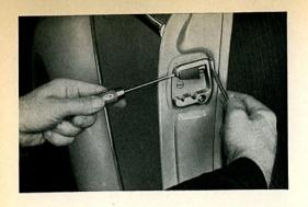
21/31 The closing pressure is regulated by adjusting the plastic wedge. After loosening the lock nut, the adjusting screw is turned with a screwdriver anticlockwise if the door is loose and clockwise if the door jams. Between a quarter and half a turn is usually sufficient. Hold the adjusting screw when tightening the lock nut to prevent the adjustment of the wedge from altering.
