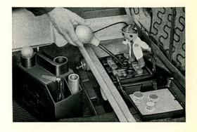
21/42 We cannot have a clear conscience about passing on the car to the Sales Department until we have examined the car from underneath. There is no need to check every nut and bolt — this is done during the 500 km (300 miles) Inspection. It is sufficient to carry out a visible check. Obviously we use tools if we discover an oil leak as indicated here by the oil strainer.
