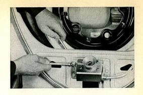
21/20 If due to maladjustment the pin is too short, it will be hard to release the lock. The hood will then require considerable pressure when closing it — a defect which will be a source of continuous annoyance to the customer later on. We can remedy this by loosing the pin nut and screwing out the pin slightly with a screwdriver.
