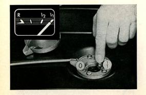
21/14 We now push the float arm forward as far as the stop. This is the position it will be in when the tank is full. This position is marked 1/1 on the picture. The gauge needle must also be on the 1/1 mark i. e., "full". Irrespective of the fuel level in the tank, a gauge set in this way will give correct readings and the customer can really rely on it.
