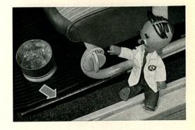
21/36 We switch on the ignition: the generator and oil pressure warning lights must come on. We start the engine: both lights should go out and thereby indicate that the generator is charging and that the oil pressure is sufficient. We depress the horn lever — the horn is in order. We must also ensure that the steering is locked when the key is removed at the "Halt" position and that the lock disengages again.
