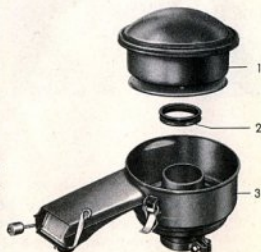
1 - Filter element, 2 - Gasket, 3 - Oil reservoir
