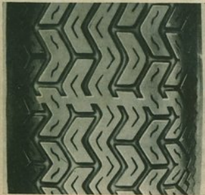
Indicator visible – tread worn
