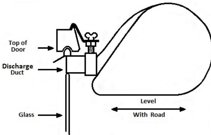
The air deflectors mounted in the discharge duct may be adjusted to direct the air to any desired portion of the automobile.
