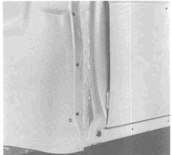
A III/6 - At the grommets for parking lamp and brake light switch cables and the seal for the speedometer drive cable in the side panel (illustration) and the lower rubber mounting for the steering column tube.
