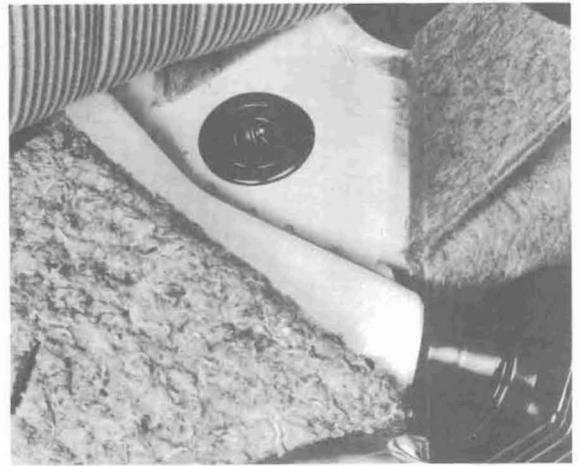
D 5 - At the welded or flanged seam where warm air pipe passes through luggage compartment floor.
