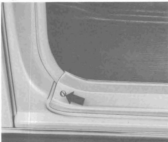
b - If necessary, coat joint between sill panel cover and outer side member with jointing compound D 20. If the cover contacts badly at the joint, it must be secured with a countersunk tapping screw (Part No. N 13 968 1).
