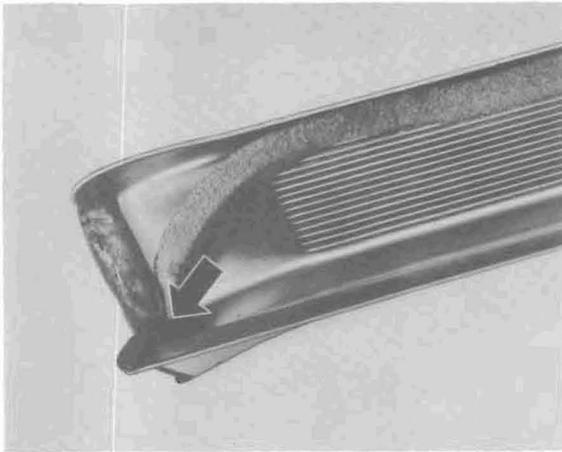
C 8 - Under the sill panel cover at front and rear, mainly at joint between plastic foam strip and door beading.
