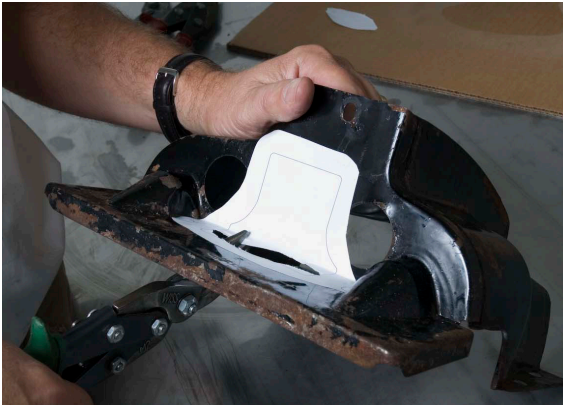
Trimming the cylinder tin.
